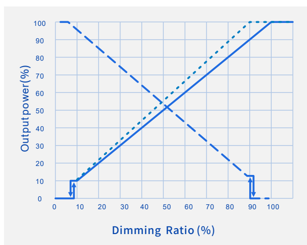
O/P Power Vs. Dimming
